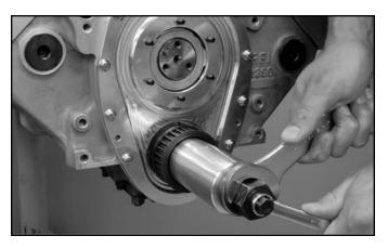
**STEP 15:** Install the crankshaft pulley using a balancer installation tool in conjunction with optional tool as shown. <u>**DO NOT</u></u> install the crankshaft pulley with a hammer or other such tool.** Verify that the crankshaft pulley does not hit the three button head cap screws used to retain the seal as mentioned in **STEP 6.**</u>
