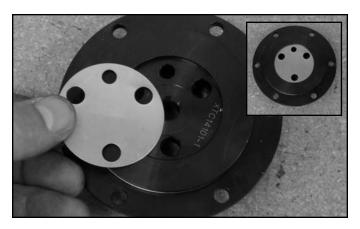
**STEP 25:** Should the cam require rearward spacing (away from the front of the engine) install the alignment shim(s) as shown and make sure that all holes in the shim(s) align with all holes in the cam drive hub **(INSET)**.
