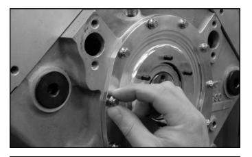
**STEP 9:** Install the back cover using the 1/4 - 20 12-point bolts provided in this kit. Bolts should only be finger tight at this step. This cover is oring sealed, **DO NOT** use a gasket when installing this cover.
