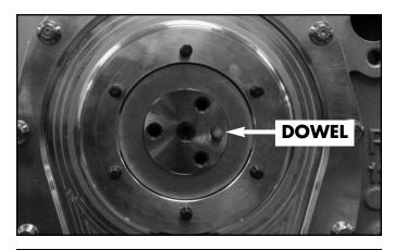
**STEP 22:** Before the camshaft thrust bearing assembly is installed, rotate the camshaft until the dowel pin is in the 3 o'clock position.
