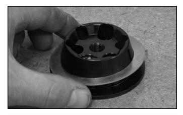
**STEP 16:** Prior to assembling the cam thrust bearing assembly, place the large I.D. copper thrust washer over the adaptor hat as shown.
