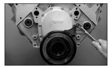
**STEP 40 (OPTIONAL):** Torque the socket head cap screws to 96 lbs/in. Set TDC as necessary. Several timing pointers are available to cover a wide range of dampers (see the front page of these instructions).
