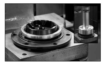
**STEP 18:** Place the seal plate and seal over the adaptor hat as shown here. Apply a thin film of Red Loctite around the OD of the seal and press in place using optional tool #CVT-CD1 (**INSET**) until the seal is flush.
