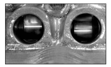
**STEP 24:** Verify camshaft alignment at this step. Alignment shims are available separately to move the cam back, towards the rear of the engine in .010", .015" and.020" increments. Shims are available to move the cam forward in .010" increments. See front page of these instructions for ordering information.
