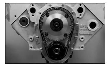
**STEP 35:** The timing marks on each pulley are for installation reference only. The cam must now be properly degreed. Once this is completed, apply Blue Loctite to the threads of each cam pulley stud and torque each of the four ARP 12-point nuts to 18 lbs-ft. Installation is complete.
