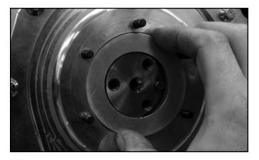
**STEP 20:** Prior to installing the camshaft drive hub assembly, the second copper thrust washer MUST be installed over the camshaft as shown. Use a small amount of grease on the back side of the washer to "stick" it to the engine. This will not affect your thrust reading.
