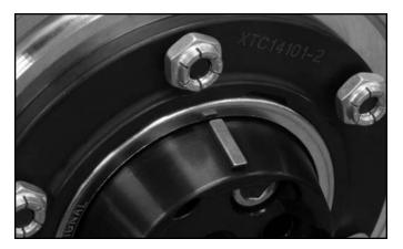
**STEP 29:** Using a small punch or brass drift and a small hammer, install the Woodruff key into the hub of the cam thrust bearing assembly. The key should be seated evenly against the bottom of the keyway slot.
