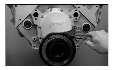
**STEP 39 (OPTIONAL):** To install the optional timing pointer, remove two of the bolts used to attach the back cover to the engine block. The mounting screws included with the pointer may be too short to use with the Xceldyne belt drive. It this is the case, substitute them for 1/4-20 x 2" socket head cap screws and install using Loctite 242 Blue threadlocker.
