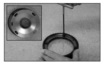
**STEP 30: FOR KITS WITH PRE-INSTALLED CAM PULLEY STUDS, GO TO STEP 31** Apply a drop of Loctite 242 Blue to the threads of the four cam pulley studs and thread them into the back sode of the cam pulley. The back side has spotfaces around each hole. The advance/retard marks are on the front side of the cam pulley (**INSET**).
