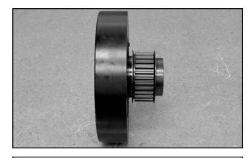
**STEP 10:** The crankshaft pulley should freely slide over and bottom out on your balancer hub. Due to varying tolerances between manufacturers, it is highly recommended that this fit is checked prior to installation of the belt drive.
