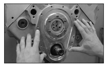
**STEP 1:** To begin, trial-fit the billet back cover to your engine block. Tolerances will vary between aftermarket block manufacturers, so some clearancing of the block may be necessary. Should this be the case with your engine, remove material from the block **NOT** from the back cover.
