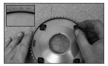
**STEP 31:** Place the spider over the studs in the cam pulley and thread the ARP 12-point nuts in place by hand. Make sure that the center degree line on the spider lines up with the mark on the cam pulley **(INSET)**.
