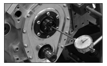
**STEP 23:** If the desired end play is not achieved using the .010" shim provided in this kit, add shims accordingly and reverify end play. Once this is achieved, a thin film of silicone sealant must be applied between all shims, the billet cover and the cam drive prior to final assembly making sure to avoid contact with the thrust washer.
