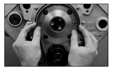
**STEP 32: NOTE -** For kits with idler bearings, stack the bearing spacer, idler bearing and washer onto the idler stud. Install the supplied 12-point nut and torque to 18 lbs-ft. - Set the cam pulley on top of the crankshaft pulley. Now slip the belt over the crankshaft pulley and over the camshaft pulley to install the belt.
