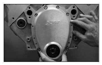
**STEP 36 (OPTIONAL):** To install the optional stamped or fabricated dust cover, choose 4 of the 10 back cover mounting bolts. In this manner, only 4 bolts have to be removed to install (or later remove) the cover. Mark the 6 bolt holes on the cover that will not be used as shown.
