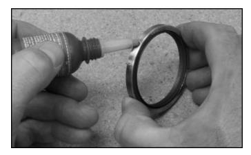
**STEP 17:** Prior to installing the camshaft seal, apply a thin, uniform coating of Loctite 272 Red to the outside diameter of the seal.
