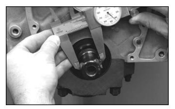
**STEP 13:** Now measure the crankshaft snout from the OD to the drive key as shown. If this measurement is larger than the measurement taken in **STEP 12**, file down the key and re-measure. Failure to verify these measurements could result in severe damage to the crankshaft pulley and/or crankshaft snout.
