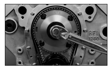
**STEP 34:** Place the camshaft pulley on to the camshaft thrust bearing assembly allowing the taper of the bearing hub to pull the camshaft pulley into position. Make certain not to dislodge the Woodruff key during this step. Install the special ARP lefthand thread retaining bolt and washer using ARP thread lube and torque to 70 lbsft.
