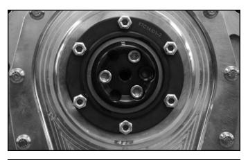
**STEP 27:** Place the camshaft thrust bearing assembly on the back cover. Install the three  $\frac{5}{16}$  - 18 socket head cap screws in the cam, then the six outer locknuts on the back cover studs as shown. Cam bolts and lock nuts should only be finger tight at this step.
