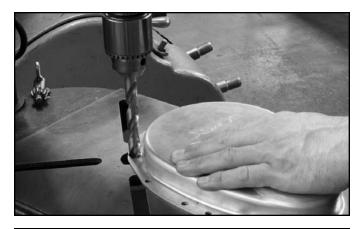
**STEP 37 (OPTIONAL):** The 6 marked bolt holes in the cover must be drilled out to  $1/2^{"}$  to allow the cover to clear the heads of the back cover bolts. Clamp the cover in a drill press or mill and drill out the holes in increments of  $3/8^{"}$ ,  $7/16^{"}$  then  $1/2^{"}$ .
