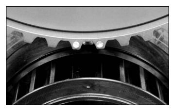
**STEP 33:** Align the timing marks on both pulleys so that the mark on the crank pulley is between the two marks on the cam pulley. **NOTE -** Kits with ialler bearings will have only one mark on the cam pulley. In this case, aligh the single mark on each pulley directly in line with each other.
