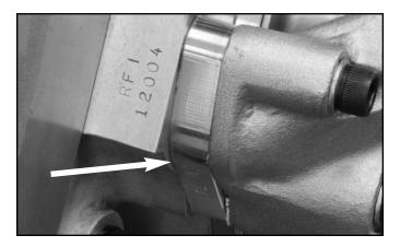
**STEP 41 (OPTIONAL):** Water pump spacers are available in a variety of thicknesses to provide clearance between the back of the water pump and the belt drive's dust cover.
