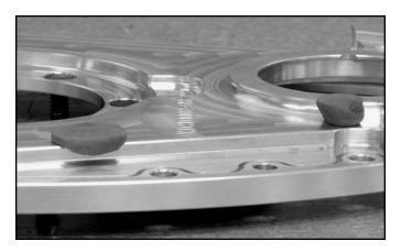
**STEP 3:** Place the back cover on the block and press against the clay. Remove the cover and inspect the clay to determine the amount of clearance between your block and the cover. Should you need to add clearance, remove material from the block **NOT** from the back cover.
