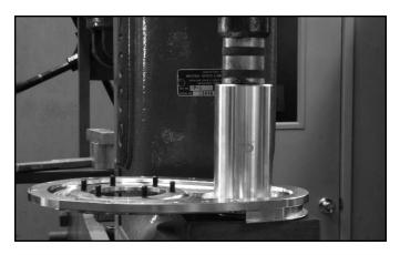
**STEP 6:** Press the crankshaft seal into the back cover using optional seal installer or similar tool. Finish the seal installation by screwing in the 3 button head cap screws provided in this kit using Loctite 242 Blue on the threads.
