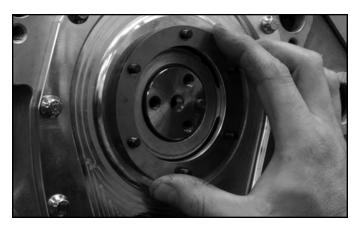
**STEP 21:** Camshaft end play must be checked before the camshaft thrust bearing assembly is permanently installed. One .005" and two .010" shims are provided in this kit for this purpose. It is recommended to use one of the .010" shims as a starting point prior to checking cam end play. Install as shown.
