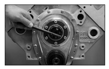
**STEP 28:** Follow the torquing sequence shown on the front page of these instructions and tighten all bolts and nuts in order, then repeat the procedure torquing them to the values listed. **IMPORTANT** - Using the optional spanner, #CVTCD3 rotate the camshaft while tightening/torquing **EACH** bolt and nut.
