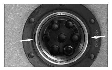
**STEP 19:** Fill the two notches in the cam thrust bearing assembly with silicone (**ARROWS**). These notches allow removal of the cam seal for maintenance and must be sealed prior to use. **NOTE - Replace thrust bearing** assembly when camshaft end-play exceeds .010".
