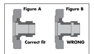
**STEP 11:** Should there be any interference in the fit of the balancer hub (shown in Figure B, exaggerated for detail) the hub OD will need to be polished or machined accordingly. Fit should be 'slip-on' with no resistance as shown in Figure A
