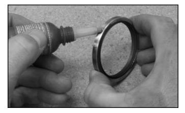
**STEP 5:** Prior to installing the crankshaft seal, apply a thin, uniform coating of Loctite 272 Red to the outside diameter of the seal.
