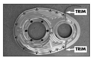
**STEP 7:** Work the o-ring cord into the dovetail groove on the back side of the cover as shown here. Trim off the excess cord flush with the end of the cover. **NOTE:** Do not use silicone sealer except as directed in **STEP 8**.
