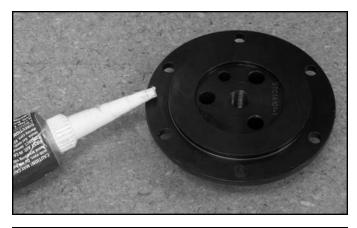
**STEP 26:** Apply a thin bead of silicone to the flange of the camshaft seal plate and smooth it out evenly with your finger.
