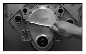
**STEP 38 (OPTIONAL): NOTE** - Deburr the 6 enlarged holes, wash the cover in solvent, dry and install. Torque the 4 mounting bolts to 96lbs/in using Loctite 242 Blue threadlocker. **NOTE** - A gasket may be necessary to provide proper clearance between the front cover and the cam drive.
