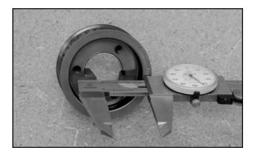
**STEP 12:** Prior to installing the crankshaft pulley, measure from the ID to the depth of the keyway as shown. Record this number.
