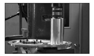
**STEP 6:** Press the crankshaft seal into the back cover using optional CV seal installer or similar tool. Finish the seal installation by screwing in the 3 button head cap screws provided in this kit using Loctite 242 Blue on the threads.
