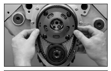
**STEP 27: NOTE -** For kits with idler bearings, stack the bearing spacer, idler bearing and washer onto the idler stud. Install the supplied 12-point nut and torque to 18 lbs-ft. - Set the cam pulley on top of the crankshaft pulley. Now slip the belt over the crankshaft pulley and over the camshaft pulley to install the belt.
