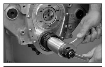
**STEP 15:** Install the crankshaft pulley using a balancer installation tool in conjunction with CV tool #CVT-CD2 as shown. **DO NOT** install the crankshaft pulley with a hammer or other such tool.
