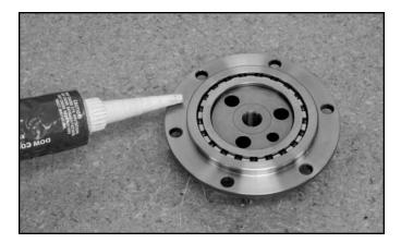
**STEP 17:** Apply a thin bead of silicone to the flange of the camshaft thrust bearing assembly and smooth it out evenly with your finger.
