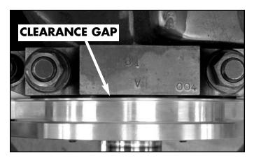
**STEP 4:** Proper oil drainback also depends on some clearance between the front main cap and back cover. Any amount of clearance is acceptable, such as shown here. Should you need to add clearance, ball mill a vertical slot in the main cap, **NOT** from the back cover.
