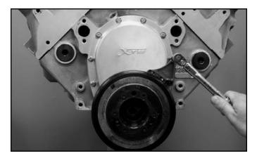
**STEP 35 (OPTIONAL):** Torque the socket head cap screws to 96 lbs/in. Set TDC as necessary. CV Products offers several pointers to cover a wide range of dampers (see the front page of these instructions).
