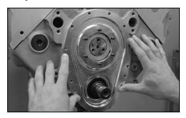
**STEP 1:** To begin, trial-fit the billet back cover to your engine block. Tolerances will vary between aftermarket block manufacturers, so some clearancing of the block may be necessary. Should this be the case with your engine, remove material from the block **NOT** from the back cover.
