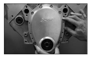
**STEP 31 (OPTIONAL):** To install the optional stamped or fabricated dust cover, choose 4 of the 10 back cover mounting bolts. In this manner, only 4 bolts have to be removed to install (or later remove) the cover. Mark the 6 bolt holes on the cover that will not be used as shown.
