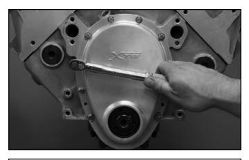
**STEP 33 (OPTIONAL): NOTE** - Deburr the 6 enlarged holes, wash the cover in solvent, dry and install. Torque the 4 mounting bolts to 96lbs/in using Loctite 242 Blue threadlocker. **NOTE** - A gasket may be necessary to provide proper clearance between the front cover and the cam drive.
