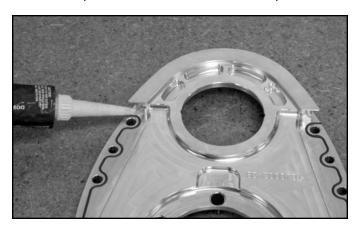
**STEP 8:** Apply a thin bead of silicone along the cover as shown. The bead should go from the o-ring to the pan seal flange.
