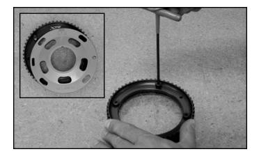
**STEP 24: FOR KITS WITH PRE-INSTALLED CAM PULLEY STUDS, GO TO STEP 25 -** Apply a drop of Blue Loctite to the threads of the four cam pulley studs and thread them into the back sode of the cam pulley. The back side has spotfaces around each hole. The Xceldyne logo is on the front side of the cam pulley (INSET).
