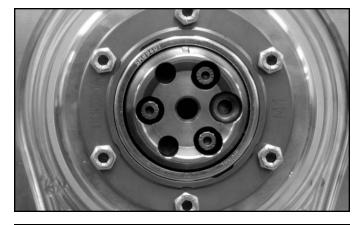
**STEP 23:** Fill the two notches in the cam thrust bearing assembly with silicone (ARROWS). These notches allow removal of the cam seal for maintenance and must be sealed prior to use. **NOTE - Replace thrust bearing assembly when camshaft end-play exceeds .010".**
