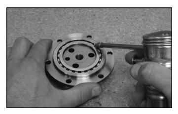
**STEP 16:** Thoroughly clean the cam thrust bearing assembly to remove all of the anti-rust agent from the assembly. Blow dry and lubricate the bearing with motor oil, rotating the thrust bearing to work the oil in evenly.
