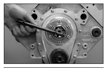
**STEP 21:** Follow the torquing sequence shown on the front page of these instructions and tighten all bolts and nuts in order, then repeat the procedure torquing them to the values listed. **IMPORTANT -** Using the optional spanner, CV tool #CVT-CD3 rotate the camshaft while tightening/torquing **EACH** bolt and nut.
