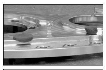
**STEP 3:** Place the back cover on the block and press against the clay. Remove the cover and inspect the clay to determine the amount of clearance between your block and the cover. Should you need to add clearance, remove material from the block **NOT** from the back cover.
