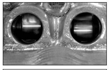
**STEP 20:** Verify camshaft alignment at this step. Alignment shims are available separately from CV Products to move the cam back, towards the rear of the engine in .010", .015" and .020" increments. Shims are available to move the cam forward in .010" increments. See front page of these instructions for ordering information.
