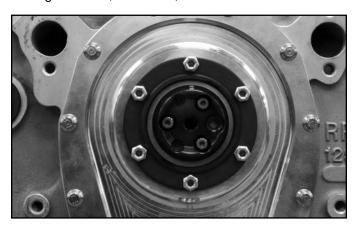
**STEP 19:** Place the camshaft thrust bearing assembly on the back cover. Install the three ARP  $^5/_{16}$  - 18 12-point bolts in the cam, then the six outer locknuts on the back cover studs as shown. Cam bolts and lock nuts should only be finger tight at this step.
