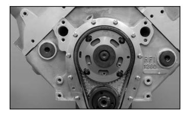
**STEP 30:** The timing marks on each pulley are for installation reference only. The cam must now be properly degreed. Once this is completed, apply Blue Loctite to the threads of each cam pulley stud and torque each of the four ARP 12-point nuts to 18 lbs/ft. Installation is complete.
