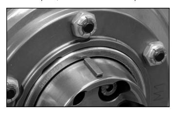
**STEP 26:** Using a small punch or brass drift and a small hammer, install the Woodruff key into the hub of the cam thrust bearing assembly. The key should be seated evenly against the bottom of the keyway slot.
