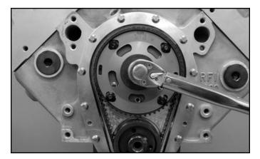
**STEP 29:** Place the camshaft pulley on to the camshaft thrust bearing assembly allowing the taper of the bearing hub to pull the camshaft pulley into position. Make certain not to dislodge the Woodruff key during this step. Install the special ARP lefthand thread retaining bolt and washer using ARP thread lube and torque to 70 lbsft.
