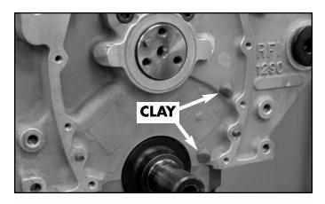
**STEP 2:** Next, check for clearance between the back cover and engine block to allow proper oil drainback. Place a small piece of clay on the highest points on the block as shown here (for example only, block designs will vary).
