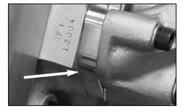
**STEP 36 (OPTIONAL):** CV Products carries water pump spacers to in a variety of thicknesses to provide clearance between the back of the water pump and the belt drive's dust cover.
