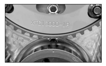
**STEP 28:** Align the timing marks on both pulleys so that the mark on the crank pulley is between the two marks on the cam pulley. **NOTE -** Kits with idler bearings will have only one mark on the cam pulley. In this case, align the single mark on each pulley directly in line with each other.
