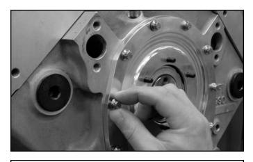
**STEP 9:** Install the back cover using the ARP 1/4 - 20 12-point bolts provided in this kit. Bolts should only be finger tight at this step. This cover is o-ring sealed, **DO NOT** use a gasket when installing this cover.
