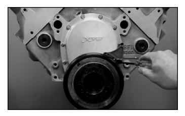
**STEP 34 (OPTIONAL):** To install the optional CV timing pointer, remove two of the bolts used to attach the back cover to the engine block. The mounting screws included with the pointer may be too short to use with the Xceldyne belt drive. If this is the case, substitute them for \$1/4.20 \times 2"\$ socket head cap screws and install using Loctite 242 Blue threadlocker.
