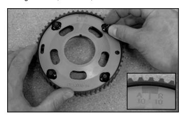
**STEP 25:** Place the spider over the studs in the cam pulley and thread the ARP 12-point nuts in place by hand. Make sure that the center degree line on the spider lines up with the mark on the cam pulley **(INSET)**.
