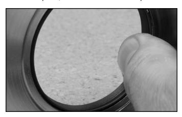
**STEP 14:** Using your thumb or finger trace the ID of the seal while applying mild pressure. this relaxes the seal allowing for easier installation of the crankshaft pulley.
