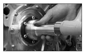
**STEP 22:** Apply Loctite 271 Red to the outer diameter of the seal as shown in **STEP 3**, then gently slide the seal up the taper of the camshaft adaptor hat until it makes contact with the seal plate. Using optional CV tool #CVT-CD1, tap the seal in place until the top of the seal is flush with the camshaft seal plate.
