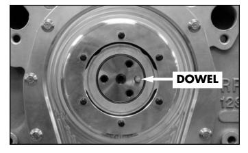
**STEP 18:** Before the camshaft bearing assembly is installed, rotate the camshaft until the dowel pin is in the 3 o'clock position.
