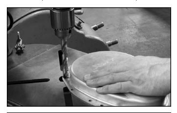
**STEP 32 (OPTIONAL):** The 6 marked bolt holes in the cover must be drilled out to  $^1/_2$ " to allow the cover to clear the heads of the back cover bolts. Clamp the cover in a drill press or mill and drill out the holes in increments of  $^3/_8$ ",  $^7/_{16}$ " then  $^1/_2$ ".
